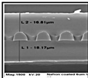
Micrographs of Giner's Dimensionally Stable Membrane
