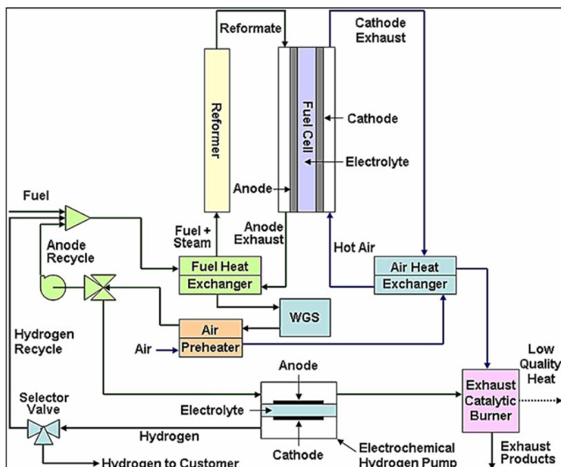
Flow Diagram of Bloom Energy's SOFC System
