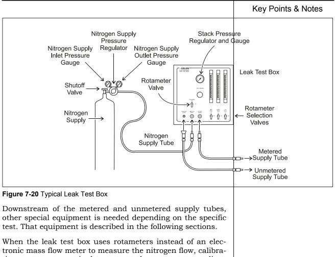
tronic mass flow meter to measure the nitrogen flow, calibration curves are required to convert the rotameters readings to flow units of cc/min. These curves are derived through experiment using standard calibration procedures. Published calibration curves are valid only for the specific rotameter, pressure and gas composition indicated. A sample calibration curve is shown in Figure 7-21. When referring to a calibration curve:
