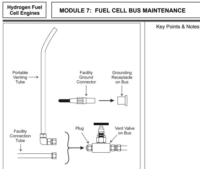
Figure 7-11 Typical Venting Equipment
