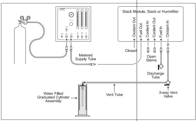
Figure 7-29 Fuel to Oxidant Transfer Leak Test
