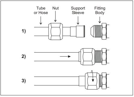
Figure 7-1 Fastening Flared Tube Fittings
