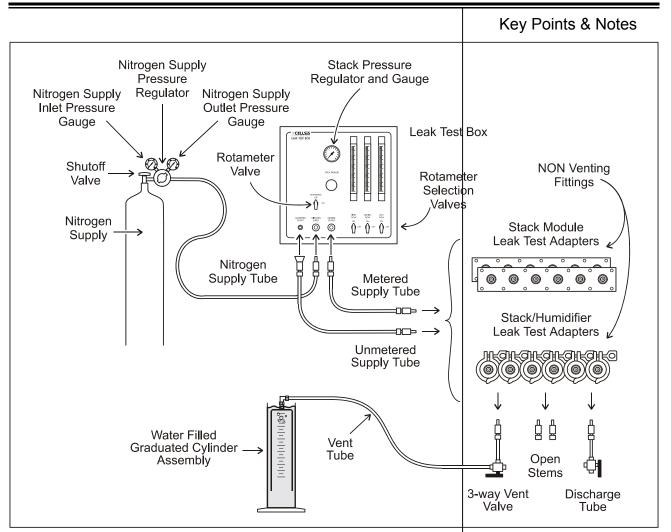
Figure 7-28 Typical Transfer Leak Test Equipment
