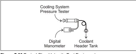
Figure 7-30 Typical Glycol Integrity Test Equipment
