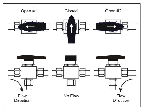
Figure 7-6 Three-Way Valve Use
