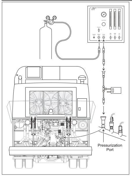
Figure 7-23 Leak-Down Test
