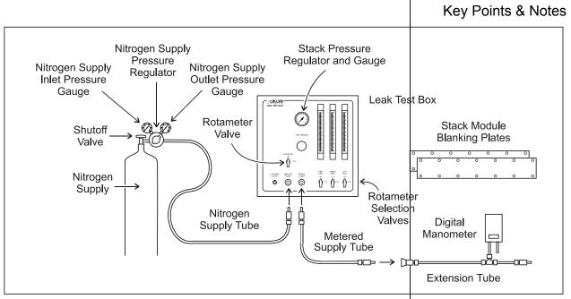
Figure 7-22 Typical Leak-Down Test Equipment
