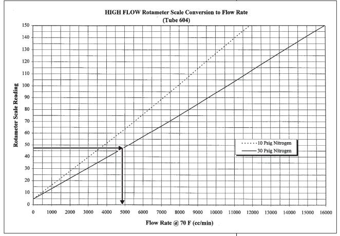
Figure 7-21 Typical Rotameter Calibration Curve
