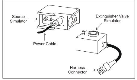
Figure 7-43 Typical Fire Suppression System Test Equipment
