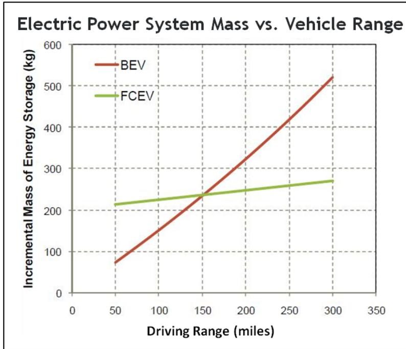
**Figure 2.2.7. Range and Mass of Energy Storage Systems for Battery Electric Vehicles (BEVs) and Fuel Cell Electric Vehicles (FCEVs)**<sup>36</sup> Battery system mass is preferable for short driving ranges (<150 miles), but FCEVs have much lower system mass (including the fuel cell and hydrogen storage systems) at longer driving ranges.
