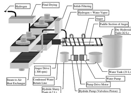
Deliverable: 50-kW prototype of a hydride hydrogen-fueled PEM fuel cell system (03/00)
