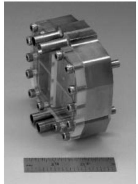
In 1999, we are demonstrating a microchannel steam-reforming reactor and microchannel recuperative heat exchangers. If the complete fuel-processing system can be miniaturized in this manner, we anticipate that the system would be smaller than one cubic foot in volume.
