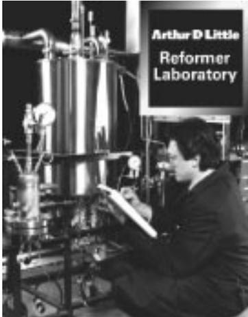
Epyx Corporation, a wholly-owned subsidiary of Arthur D. Little, Inc. (ADL), is developing a 50-kWe fuel-flexible fuel processor capable of processing gasoline and alternative fuels, such as ethanol. Major technical issues to be addressed in this program include the following: advanced catalysts, CO cleanup, transient controls, and reformer start-up/shut-down time.
