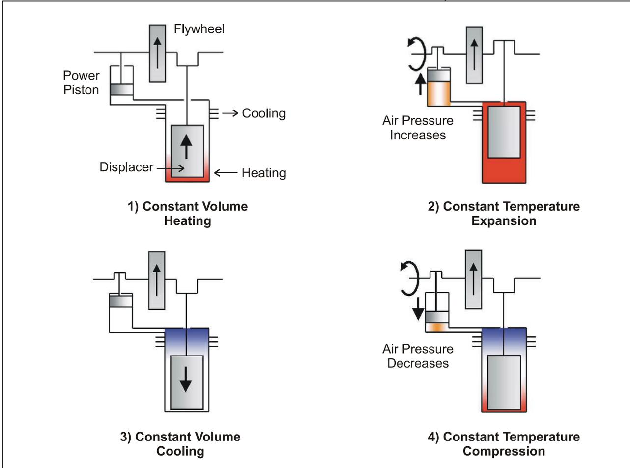
**Figure 8-9** Stirling Engine Operation
