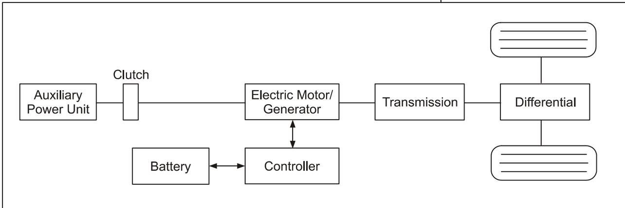
Figure 8-3 A schematic of a Parallel HEV
