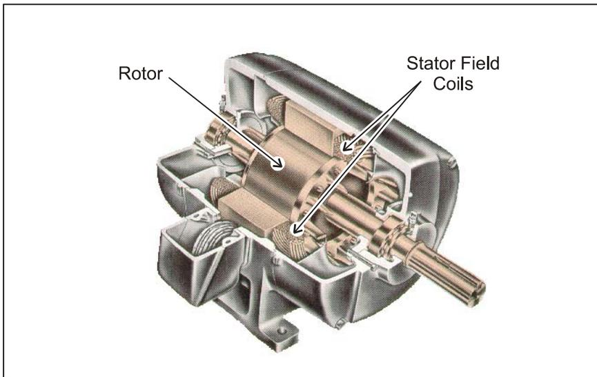
**Figure 8-5** Alternating Current Induction Motor
