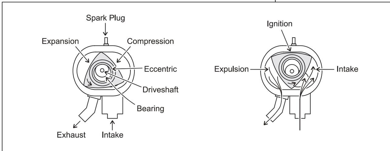
Figure 8-8 Wankel (Rotary) Engine Operation
