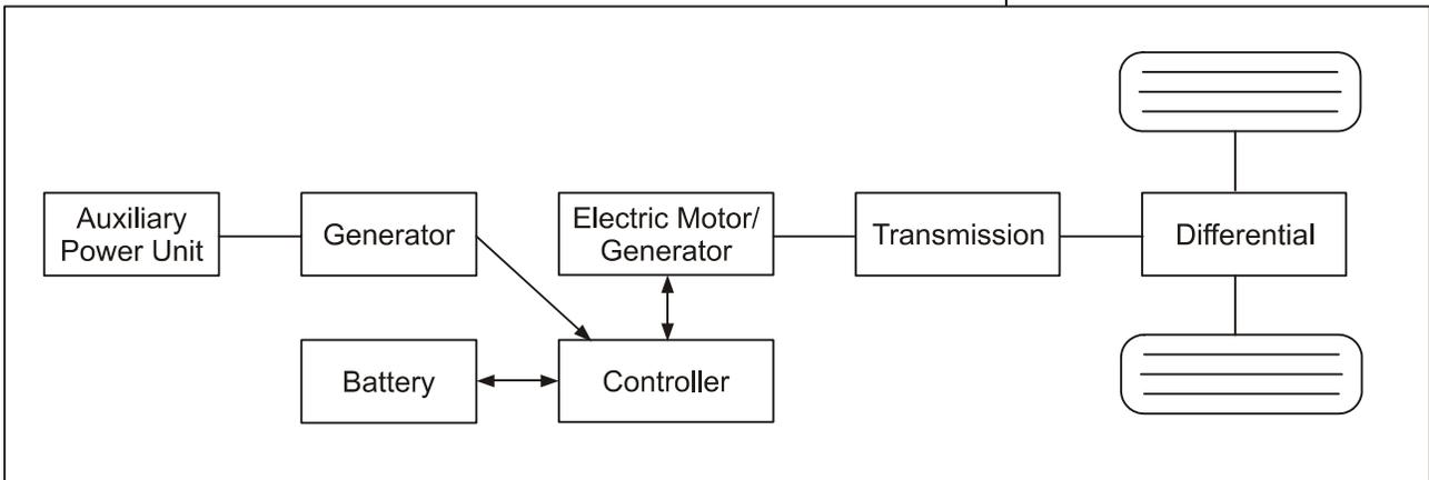
Figure 8-2 Schematic of a Series HEV
