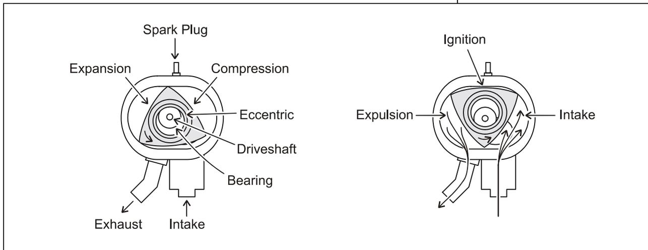
Figure 8-8 Wankel (Rotary) Engine Operation
