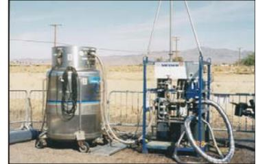
*Liquid Hydrogen Filling Tank*
