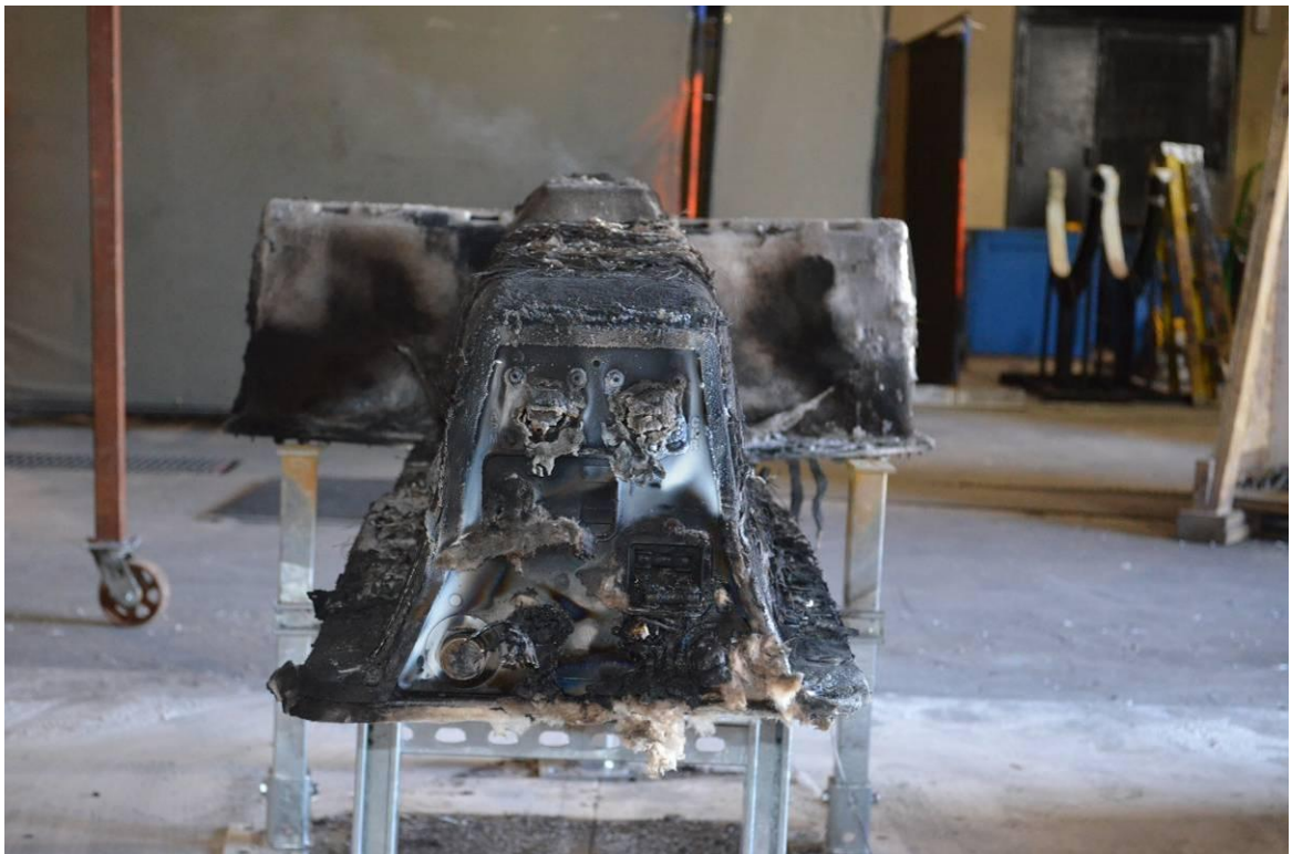
Figure A-14. Post-Test View of Battery.
