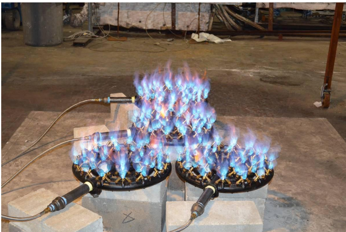
Figure 2. Propane Burners Setup Prior to Testing.
