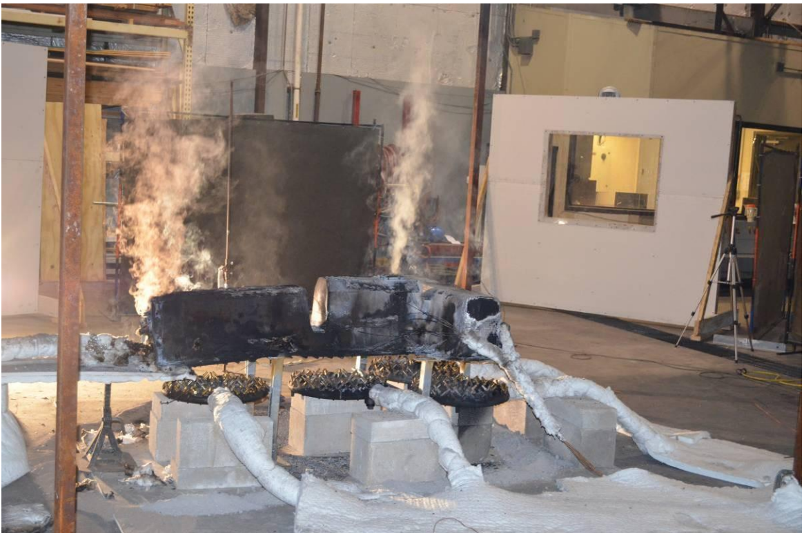
Figure A-12. Post Test View of Battery (Immediately Post Test).
