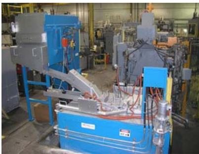
Figure 1: Contech Squeeze Casting Cell
