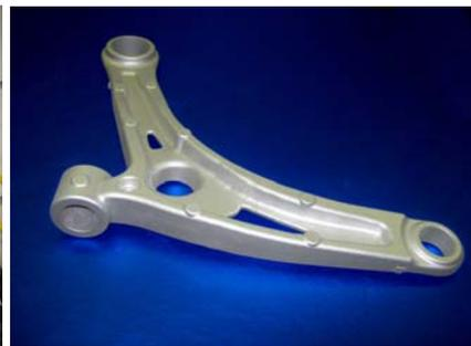
Figure 3: Magnesium Front Lower Control Arm
