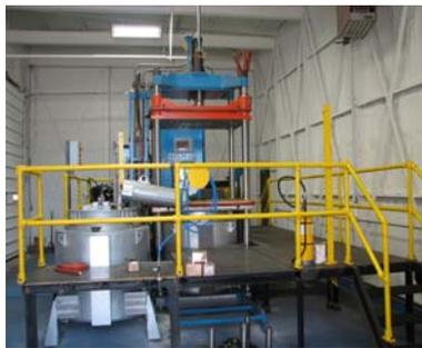
Figure 2: CMI E&E Low Pressure Casting Cell
