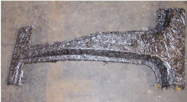
Figure 1: Carbon fiber preform for B-pillar outer panel.
