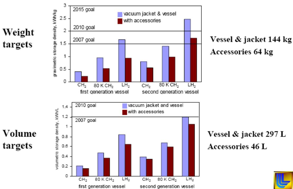
Figure 1: Weight and volume estimates for first and second generation tanks
