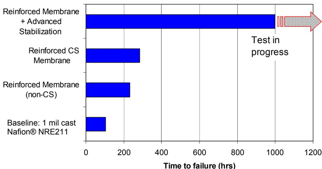
Figure 1: Accelerated durability test results: combined humidity cycling and load operation of DuPont membranes
