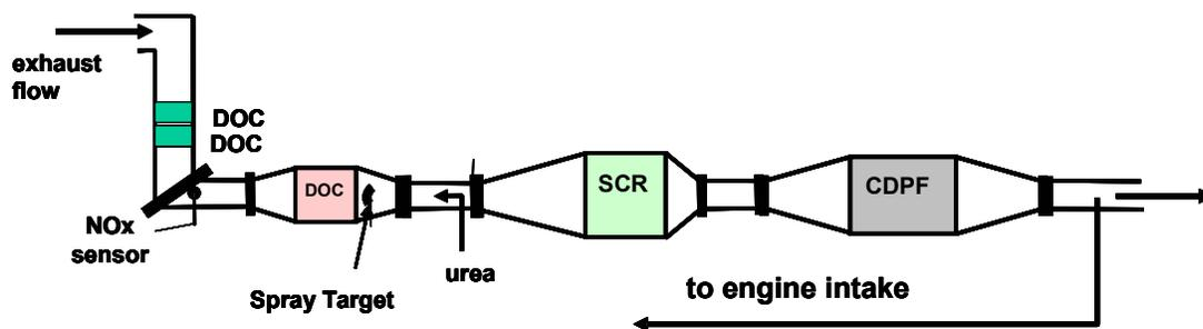
Schematic of aftertreatment system tested
