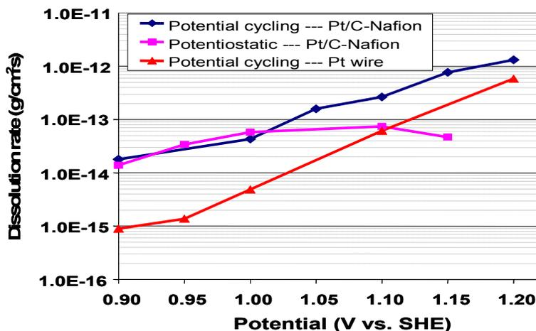
Figure 1: Effect of potential and potential cycling on Pt dissolution rate
