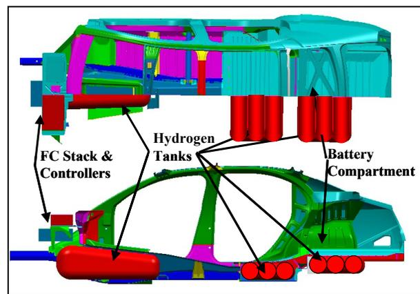
Figure 2: Fuel Cell Powertrain Components Comprehended
