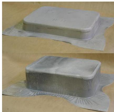
Figure 2: Deep-drawn panels warm-formed using a purpose-built warm-forming die.
