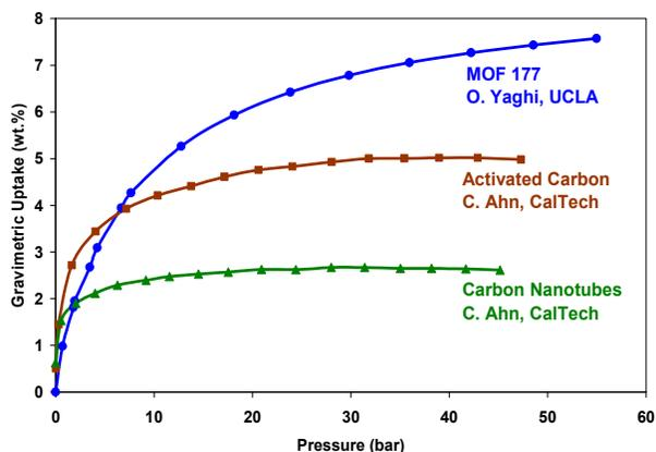
Figure 1: New engineered materials such as MOF177 by O. Yaghi (UCLA) adsorb significant amounts of hydrogen at 77°K.
