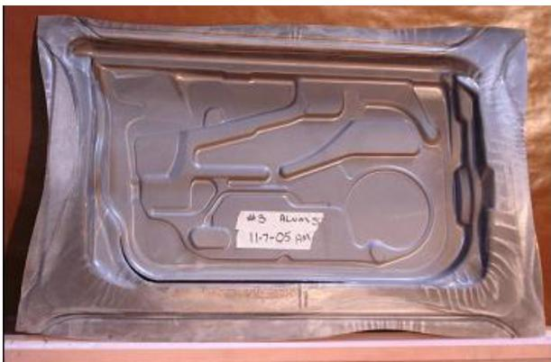
Figure 1: Inner door panel warm-formed using refitted steel-stamping die.
