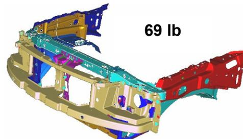
Figure 3: Conventional steel front-end structure (2006 Ford Expedition)
