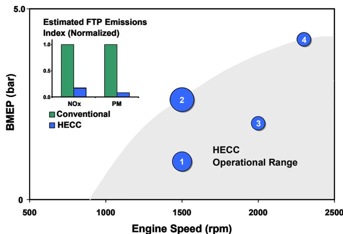
Four non-idle test conditions used in FTP simulation of a small car and normalized cycle-weighted emissions for NO<sub>x</sub> and PM for both conventional and high-efficiency modes.
