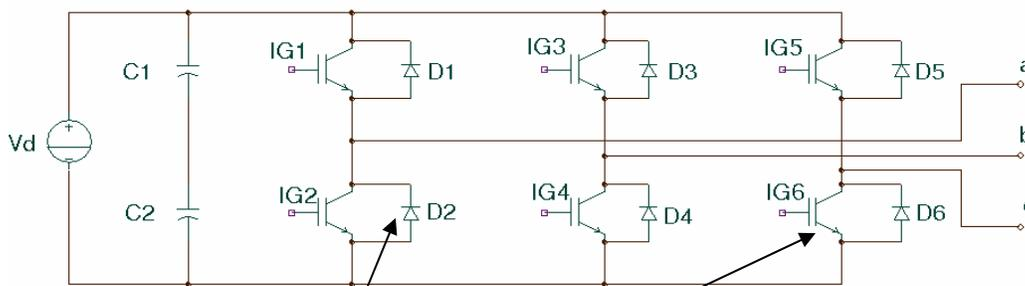
SiC Schottky Diodes (D1, D2, D3, D4, D5, D6)
