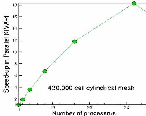
Three-dimensional representation of engine geometry used in KIVA calculations (left). A parallel-processor version of KIVA reduced calculation time by a factor of 1 to 18 depending on the number of processors used (right).
