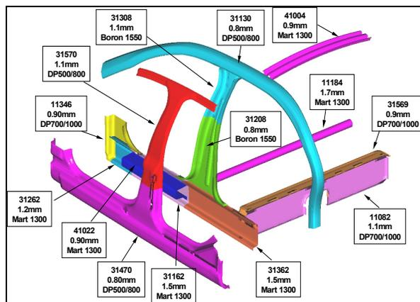
Figure 1: Optimized Advanced High Strength Steel Solution
