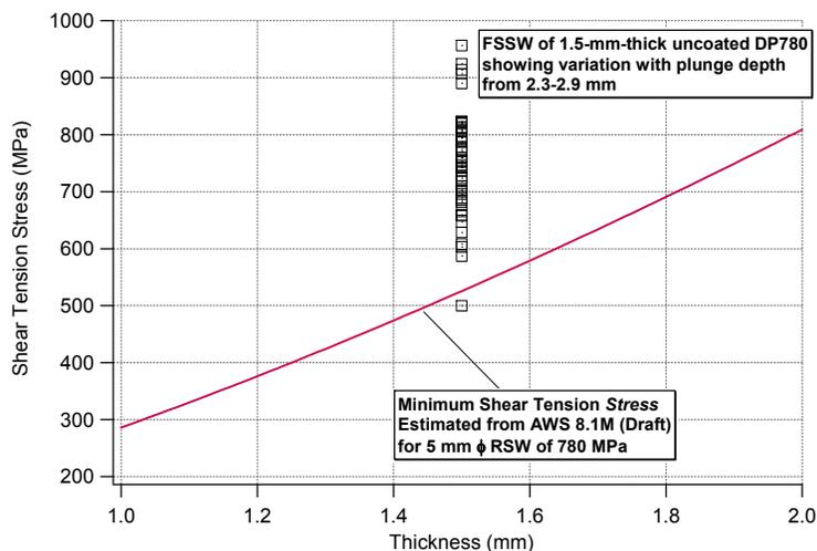
Figure 1: Variation of shear tension stress with DP780 sheet thickness. The data indicate that the intrinsic strength of FSSWs exceeds the minimum specified for RSWs.
