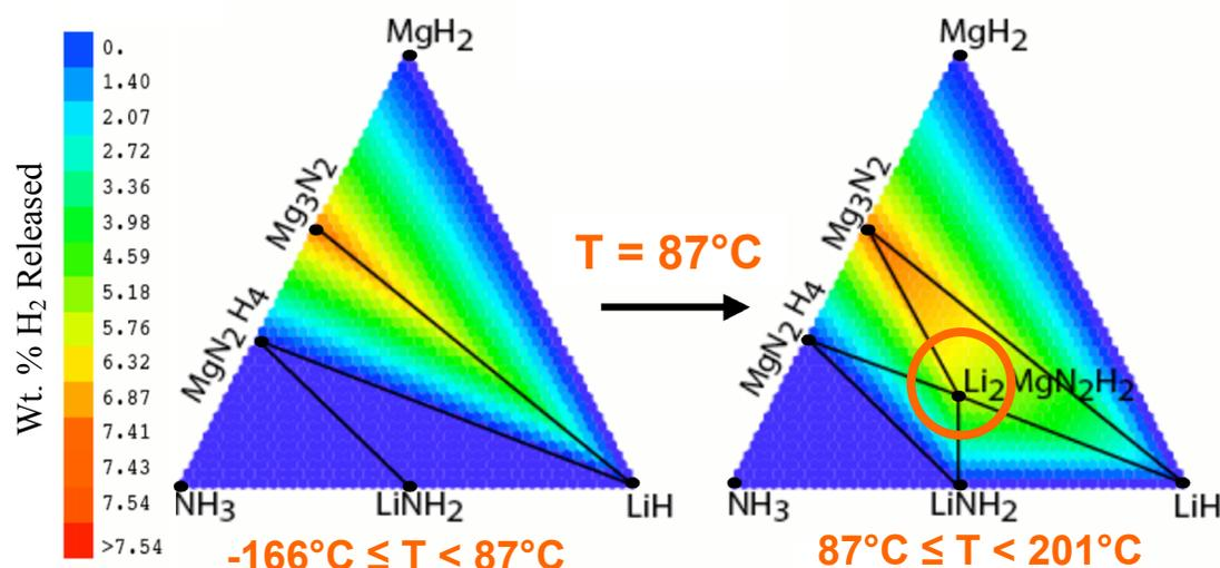
Figure 1: Calculated phase diagrams and weight percent hydrogen released for the reaction  $2 \text{LiH} + \text{Mg}(\text{NH}_2)_2 \rightarrow \text{Li}_2\text{Mg}(\text{NH})_2 + 2 \text{H}_2$  at  $T = 87^{\circ}\text{C}$  in the quaternary Li-Mg-N-H system. The appearance of the  $\text{Li}_2\text{Mg}(\text{NH})_2$  phase within the yellow-shaded region in the right diagram (circled) indicates that 5.6 wt.% hydrogen will be released at those compositions.
