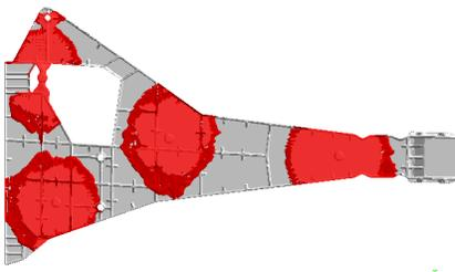
Figure 2: Flow simulation showing start of filling pattern for hot runners, as the part is filled simultaneously in four locations
