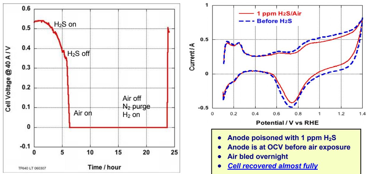
Figure 1: Air Effect on Anode Due To Shut-down
