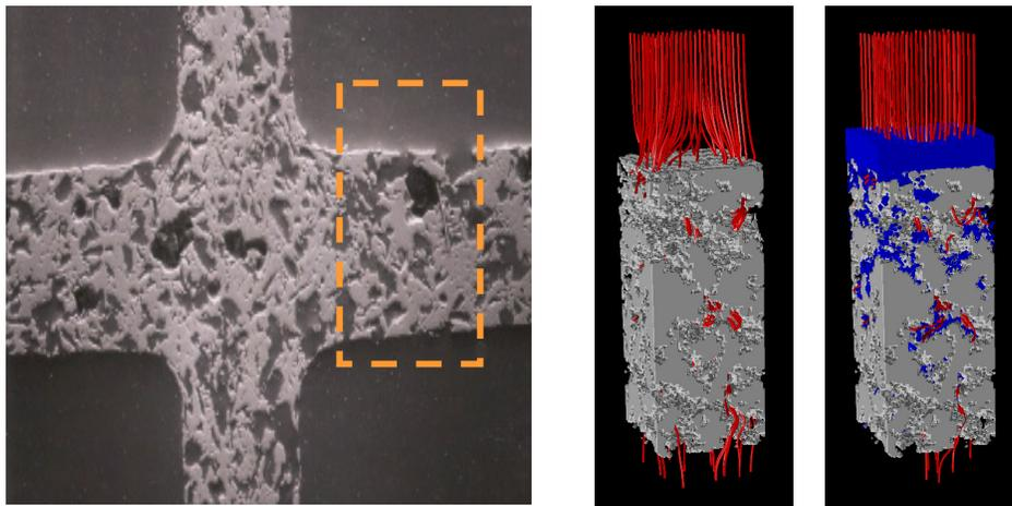
Electron microscope image of porous wall separating flow channels in a DPF. Exhaust gas flows through one channel, through the wall, and into the adjacent channel (left). Calculated flow streamlines (red) in a clean wall section (center). Calculated flow streamlines and collected soot (blue) in a wall section with soot loading.
