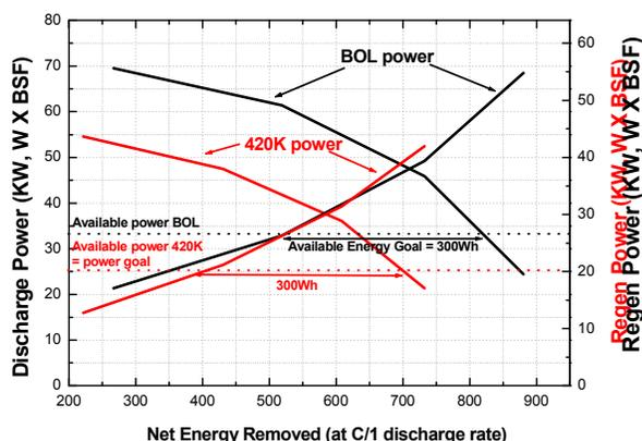
Figure 2: Energy vs. Power for G4.0 @ BOL & EOL (420,000 cycles). G4.1 & 4.1.1 tests in process are trending similarly or better than G4.0.
