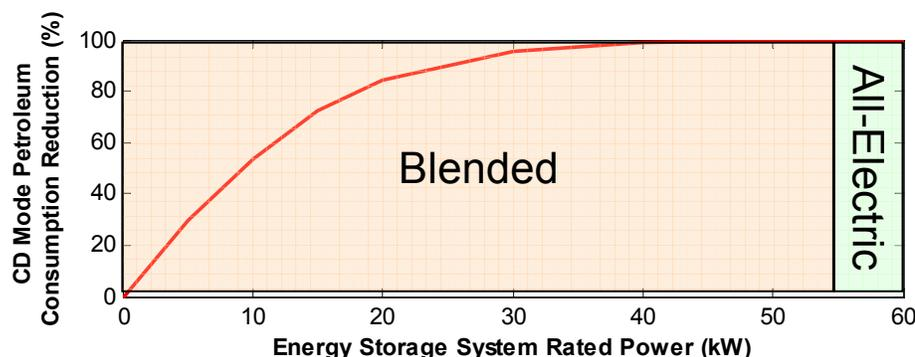
Figure 1: Petroleum Reduction vs. Battery Power during Charge Depleting Mode
