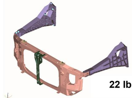
Figure 4: ULC cast magnesium front-end proposal (68% less weight)
