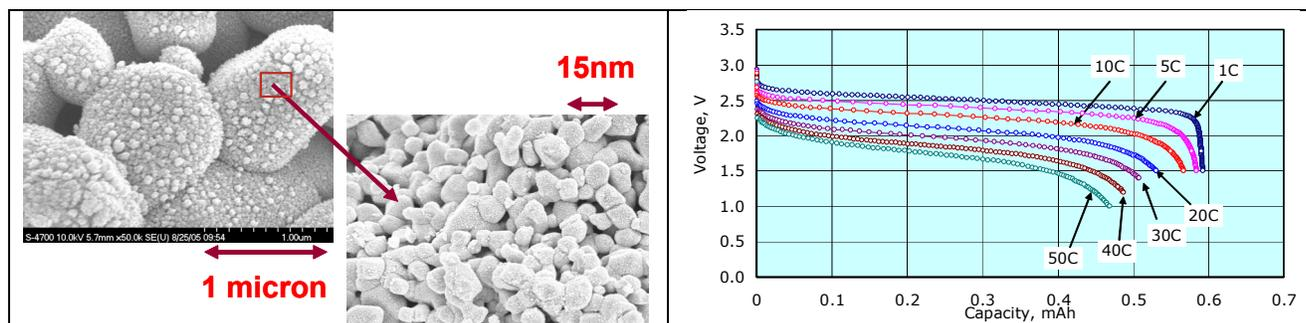
Figure 1: Cells incorporating Argonne's nano-phase lithium titanate material exhibit extremely high rate capability when coupled with lithium manganese spinel cathode.
