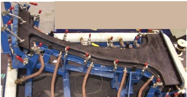
Figure 2: Carbon fiber B-pillar inner and outer panel in bonding fixture.
