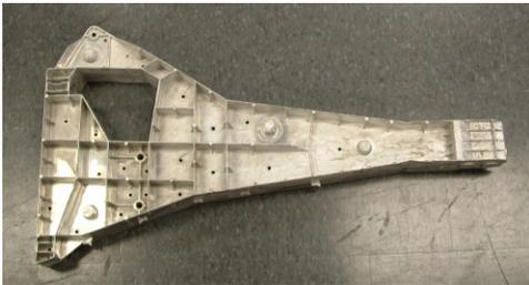
Figure 1: Thixomolded magnesium shotgun casting
