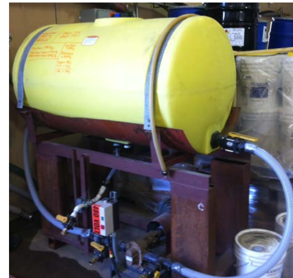
Slurry Mix Tank
