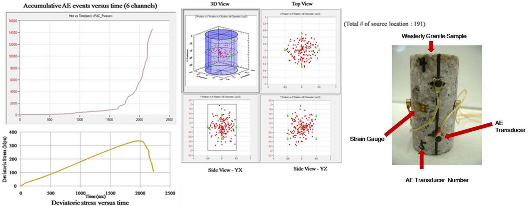
**Westerly granite sample #2** was tested under the conditions of 10 MPa confining pressure, 0.02%/min strain rate and 6-channel AE monitoring. Stress versus time curve and corresponding accumulative AE event response are shown. Good correlation between AE signal and damage accumulation in the sample has obtained. Stress-time curve and accumulative AE events ( $P_c=5\text{MPa}$ ). AE signal for each channel ( $P_c=5\text{MPa}$ ). Data compares well with Lockner et al. (1992).
