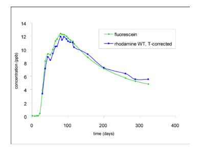
Tracer return curves from a test at Steamboat Springs involving the use of a thermally stable tracer in combination with a thermally reactive tracer.
