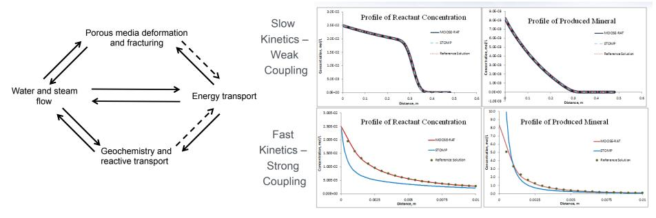
Weakly coupled processes — excellent agreement between fully-coupled and operator-split approaches Strongly coupled processes — better agreement between fully-coupled and the reference solution
