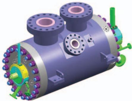
This project's team will build a prototype of the largest and highest-temperature s-CO<sub>2</sub> closed Brayton power cycle turbine ever constructed. The use of carbon dioxide instead of steam allows higher power-cycle efficiency and more compact cycle components. *Illustration from Dresser-Rand*
