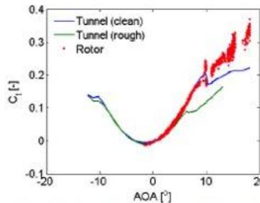
Normal force (left) and tangential force (right) coefficient vs. AOA. Blue curve is tunnel measurements on a clean airfoil, green curve is tunnel measurements on an airfoil with leading edge roughness and red dots are measurements at  $r=20m$  on the rotor.
