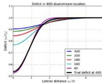
Deficits from individual turbines are compared with a more accurate solution including the wake of the upstream turbines.
