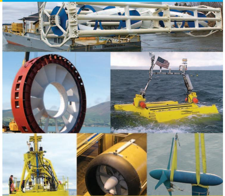
Marine and hydrokinetic devices include (clockwise from the top) Ocean Renewable Power Company's Turbine Generator Unit, NREL/PIX 17210; Columbia Power Technology's SeaRay, NREL/PIX 19381; Verdant Power's Free Flow System, NREL/PIX 17209; Free Flow Power Corporation's SmartTurbine, NREL/PIX 19382; the Wavebob point absorber, NREL/PIX 19384; OpenHydro's Open-Centre Turbine, NREL/PIX 19383
