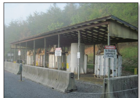
Shielded transfer tanks are stored under a shed in Melton Valley near ORNL.
