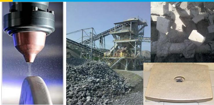
Left: Laser fusing of amorphous powders to steel component.
