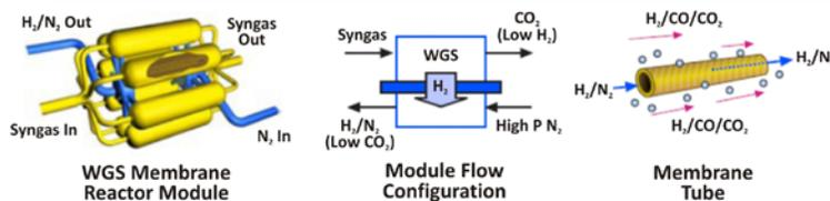
Reactor concept (left). Flow diagram (middle): Hydrogen ( $H_2$ ) permeates the membrane where nitrogen ( $N_2$ ) sweeps the gas to produce a high-pressure  $H_2/N_2$  gas stream. Membrane diagram (right): The  $H_2$ -selective membrane allows the continuous removal of the  $H_2$  produced in the water-gas-shift (WGS) reaction. This allows for the near-complete conversion of carbon monoxide ( $CO$ ) to carbon dioxide ( $CO_2$ ) and for the separation of  $H_2$  from  $CO_2$ .
