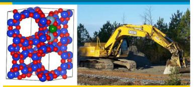
Left: Optimized structure of high-silica Cu-ZSM-5 (employing density functional theoretical methods).
