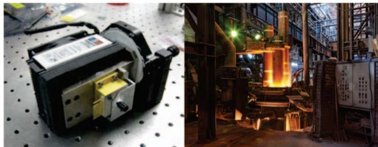
The Los Gatos Research mid-infrared laser module contains a quantum cascade laser mounted on a thermo-electric cooler (left). The Small Business Innovation Research (SBIR) Phase III analyzers will be deployed for long-term testing under industrial conditions at EAF facilities (right).
