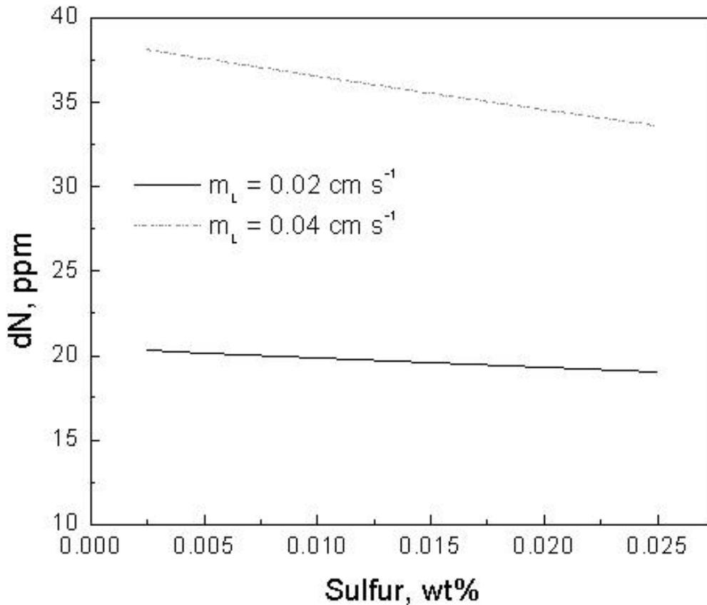
Figure 23, Nitrogen pickup for different sulfur content,  $N_i=30$  ppm,  $h_o = 0.001$
