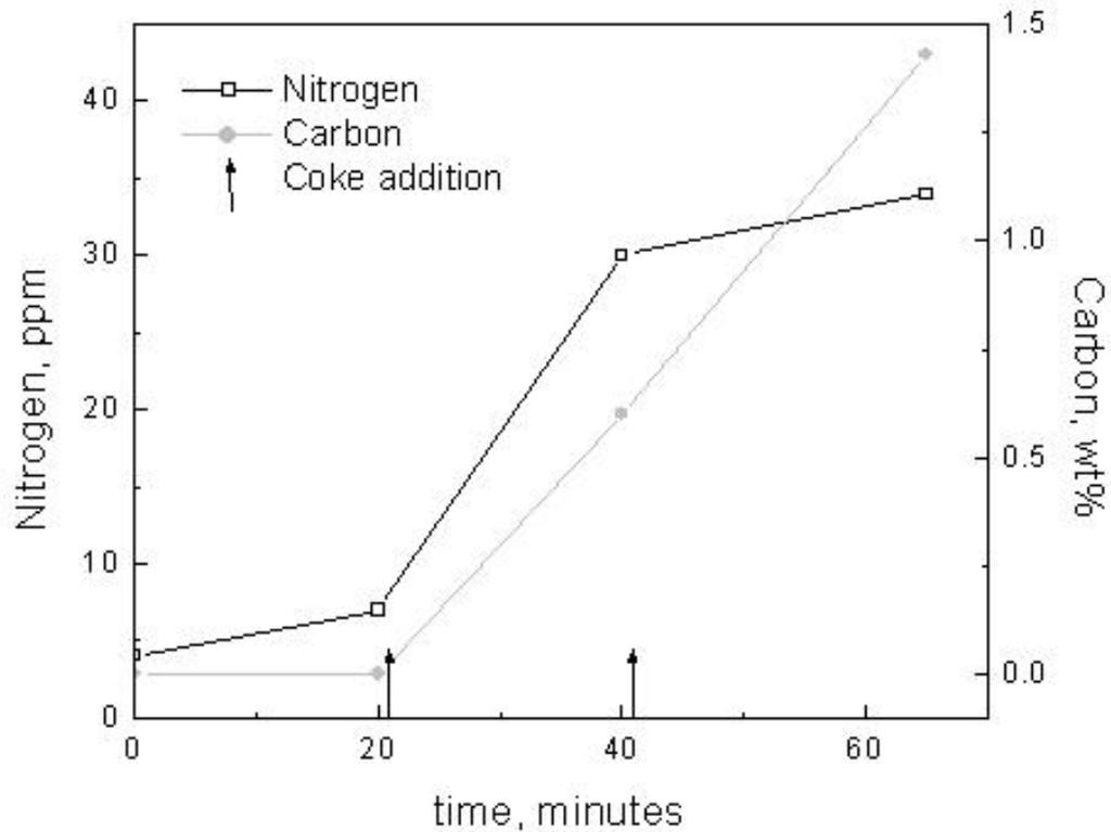
Figure 12, Effect of pitch coke (heated to 1823 K) addition on the nitrogen and carbon content of iron, Trial 5
