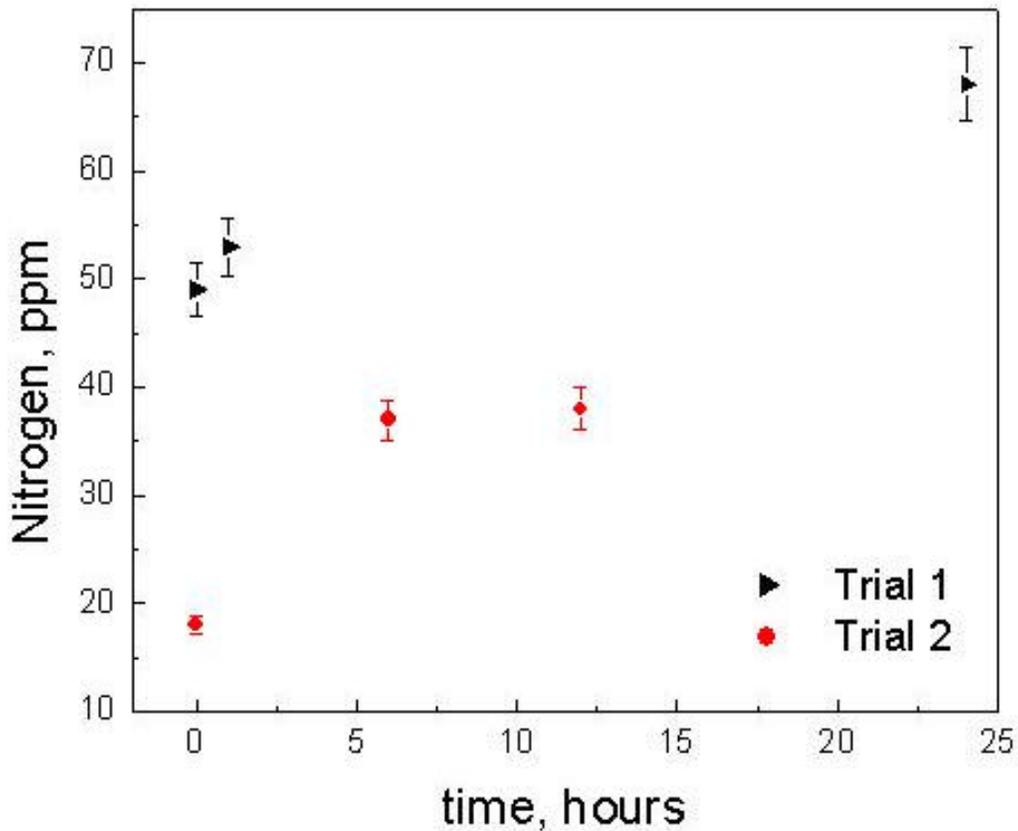
Figure 13, Nitrogen pickup through a slag layer as a function of time, Trial 1 and 2
