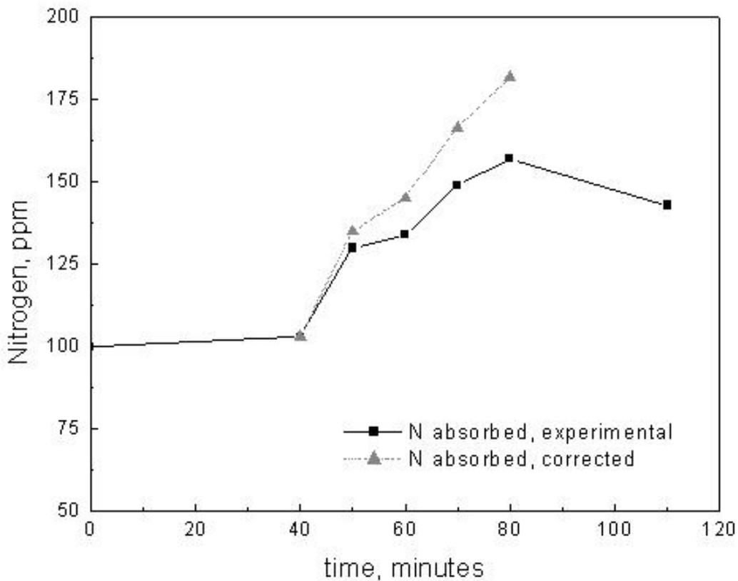
Figure 10, Nitrogen pickup corrected for the desorption, Trial 3
