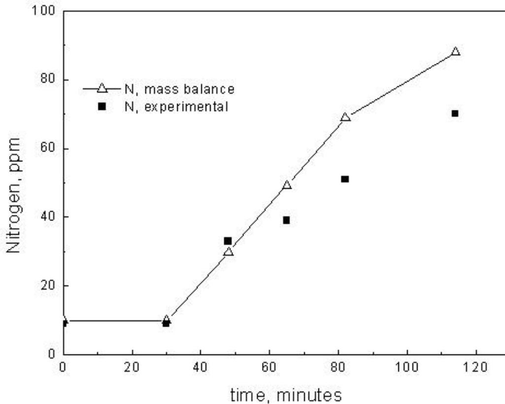
Figure 5, Nitrogen pickup from medium carbon ferromanganese, Trial 2
