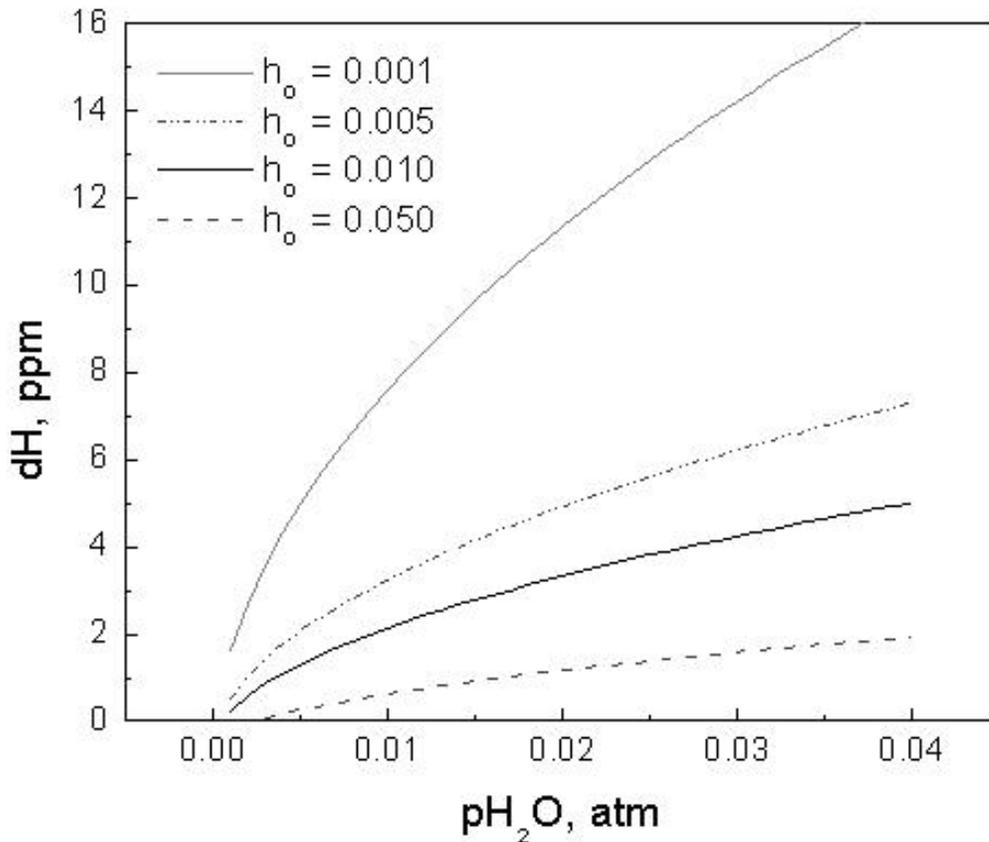
Figure 22, Hydrogen pickup for different oxygen activity at the bubble surface,  $H=3\text{ppm}$ ,  $\%S = 0.02$ ,  $m_L = 0.097 \text{ cm s}^{-1}$
