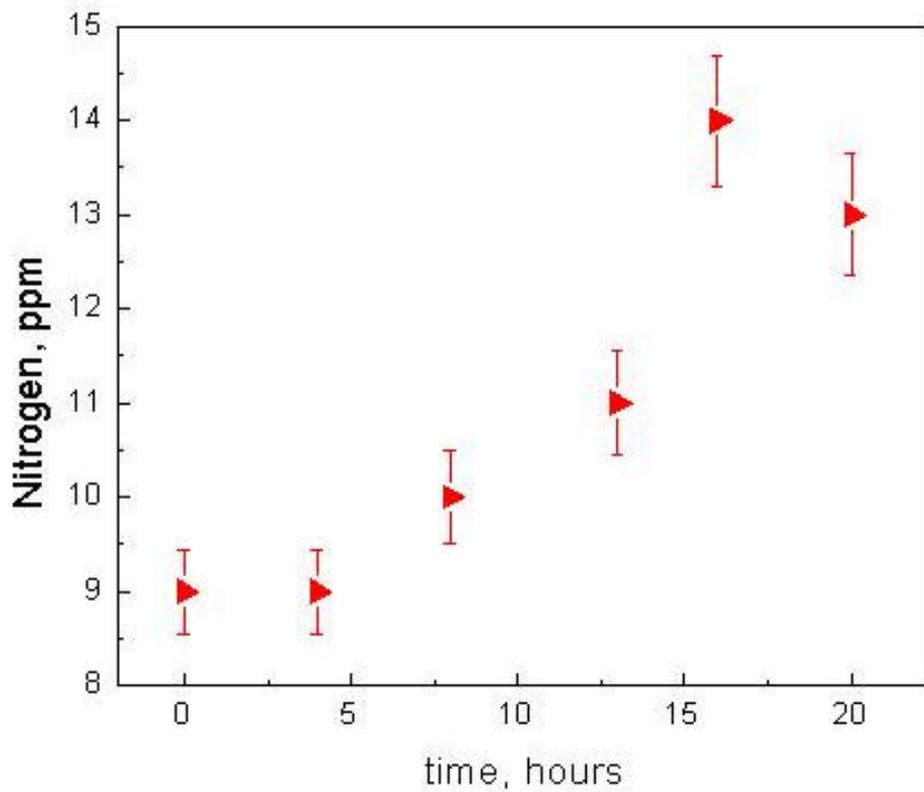
Figure 15, Nitrogen transport through MgO rich slag, Trial 3
