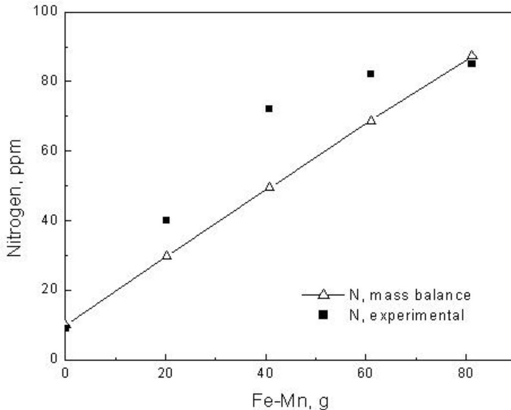
Figure 4, Nitrogen pickup from medium carbon ferromanganese, Trial 1
