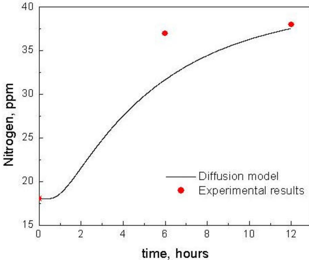
Figure 17, Nitrogen transport through slag layer, calculated and experimental, Trial 2
