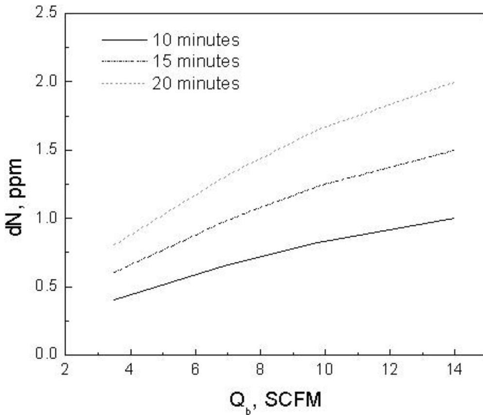
Figure 29, Nitrogen pickup at the spout eye for different stirring intervals,  $N_s = 10$  ppm, %
