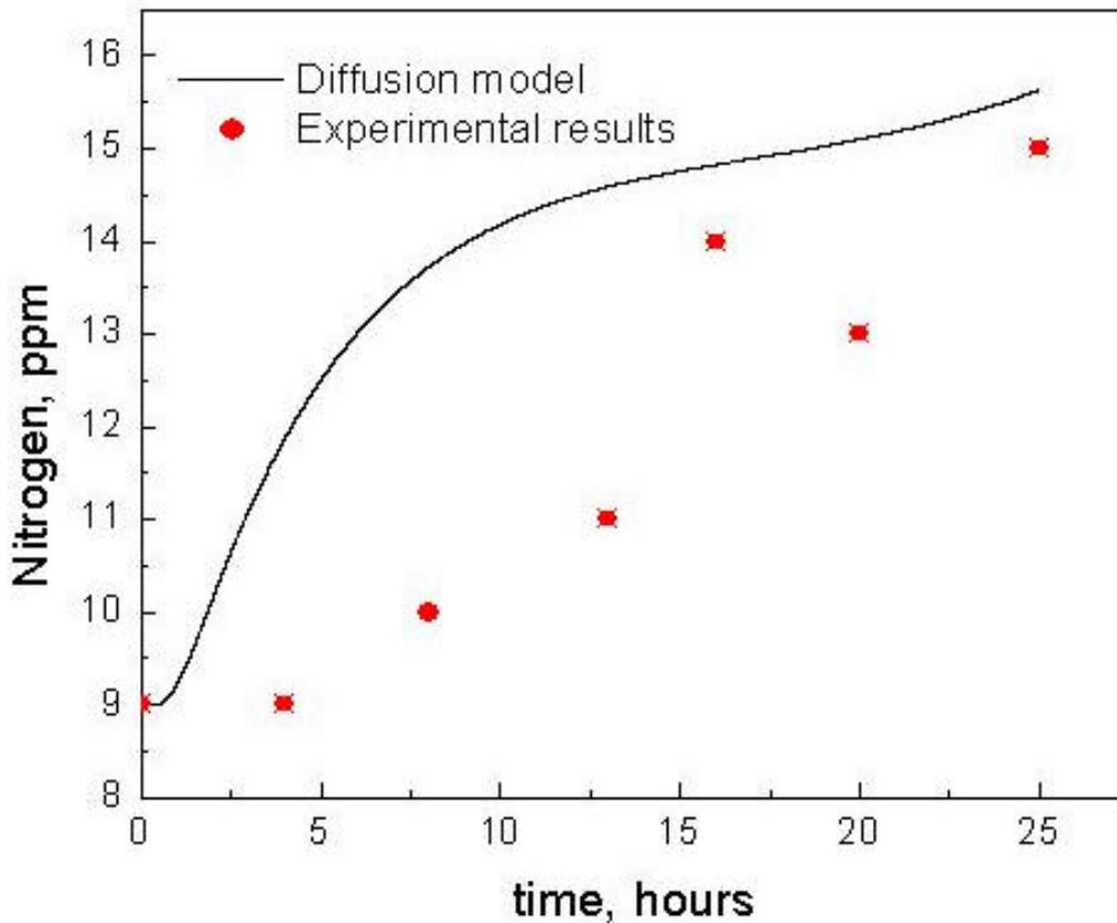
Figure 18, Nitrogen transport through slag layer, calculated and experimental, Trial 3
