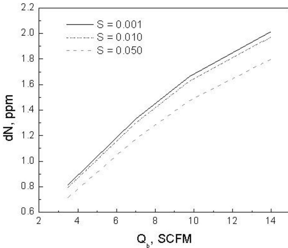
Figure 28, Nitrogen pickup at the spout eye for different sulfur concentrations,  $N = 10$  ppm,  $h_o = 0.001$ , stirring time = 20 minutes and slag thickness = 5 cm
