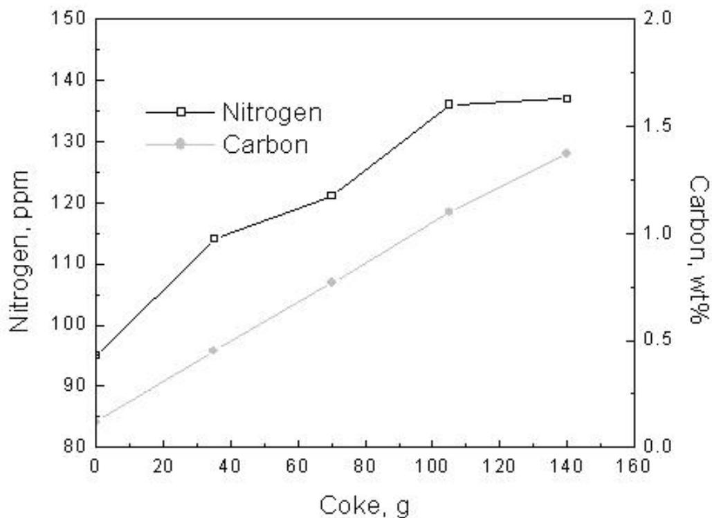
Figure 7, Effect of pitch coke addition on the nitrogen and carbon content of iron, Trial 2
