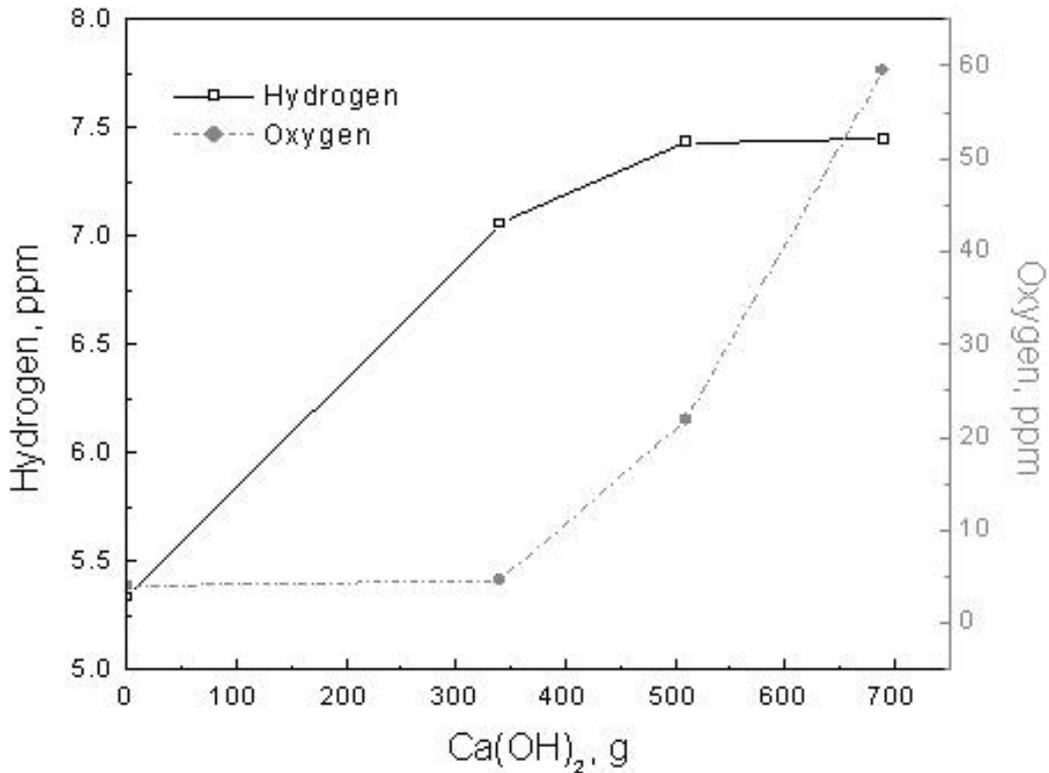
Figure 2, Hydrogen pickup due to Ca(OH)<sub>2</sub> addition along with the slag
