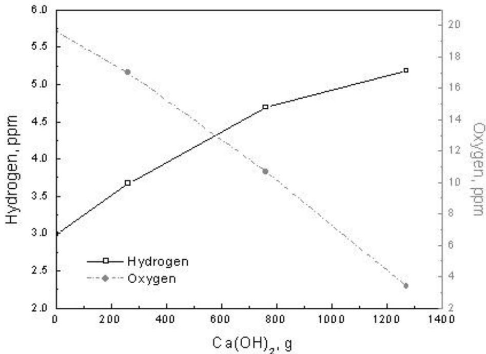
Figure 1, Hydrogen pickup due to  $\text{Ca(OH)}_2$  addition on top of the slag
