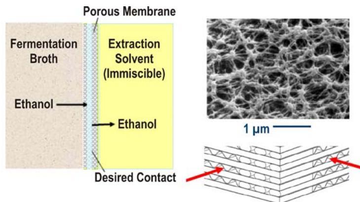
Fig1. Left – Schematic of separation of fermentation broth and a high-boiling extraction solvent using MSE. Right – Close up of microporous-membrane. By stacking layers of the membrane and incorporating integral channels, a high surface area for separation can be obtained.
