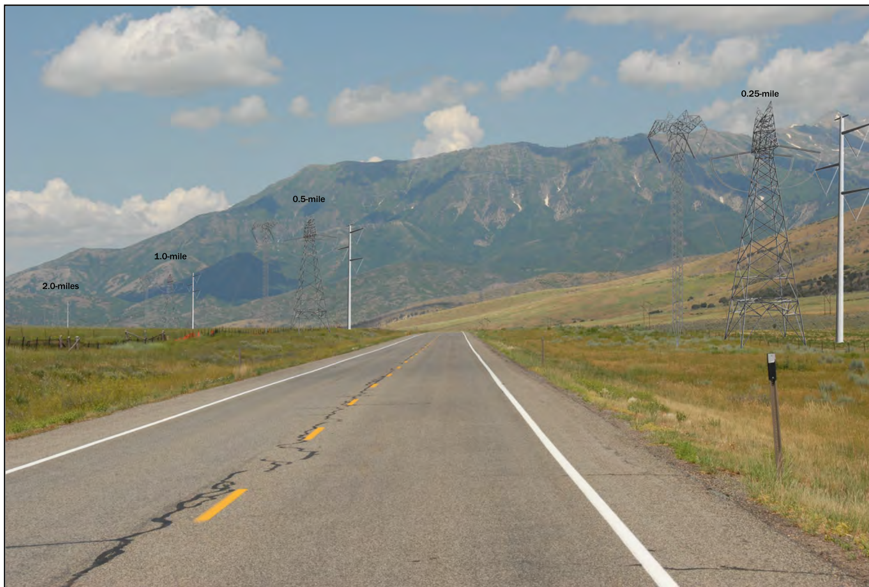
Figure 3.12-7 Comparisons of Guyed, Self-supporting, and Tubular Pole Structures at 2.0, 1.0, 0.5, and 0.25 miles with Landforms as Background
