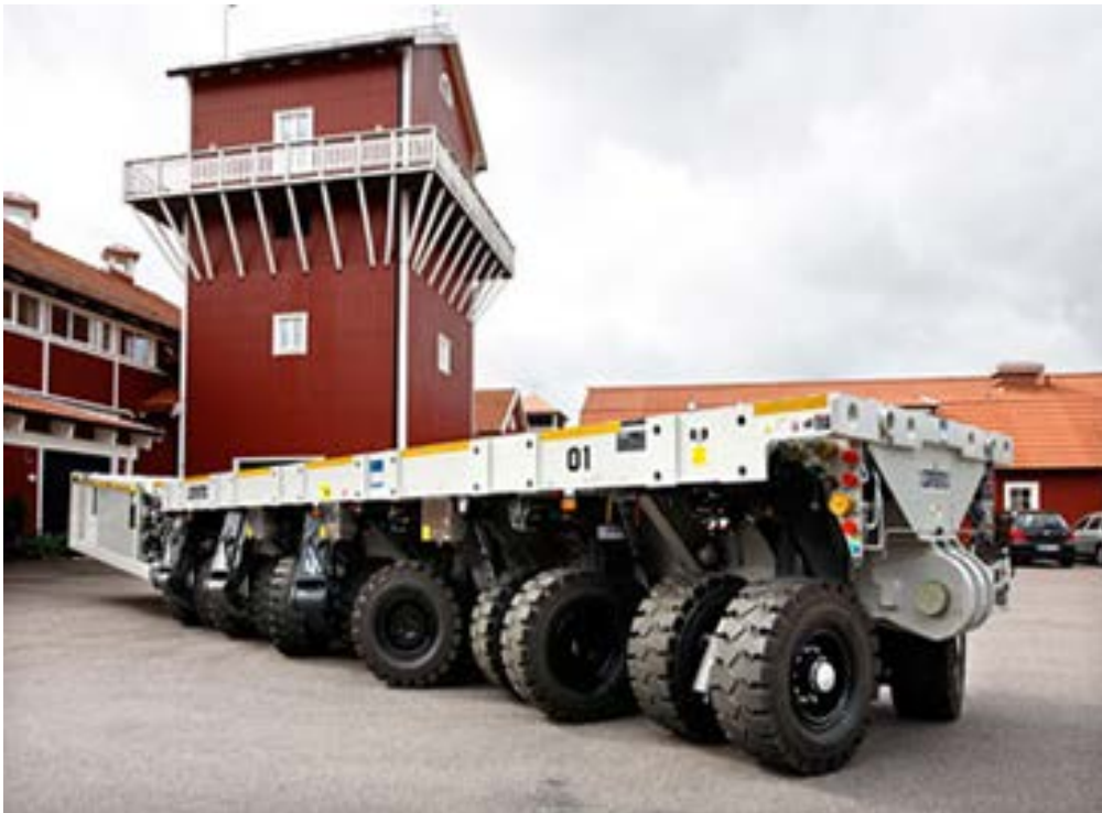
Figure 2.3-1 Diesel Powered Cometto-Built Transporter at Äspö
