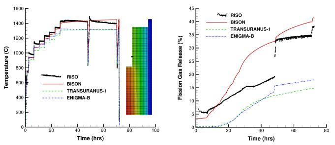
Fig. 5. Simulation of power ramp test results for the Risø AN3 experiment: (left) fuel centerline temperatures and (right) total fission gas release.
