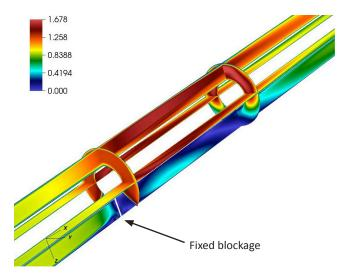
Fig. 3. Flow velocity contours from high-fidelity Nek5000 simulations of flow through the annular test section of the SIBERIA flow blockage experiment.
