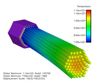
Fig. 2. Predicted deformations in the EBR-II XX09 assembly during an SHRT pseudotransient simulation. Displacements are exaggerated 100-fold. assemblies on the path to full-core multiphysics validation simulations of the EBR-II SHRT experiments. [ANL, LLNL]
