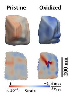
The most magnetic mineral on Earth, magnetite, cleans water contaminated by heavy metals. This process has not, up to now, been directly observed. Now, a team led by scientists from **Argonne National Laboratory** imaged the surface of magnetite and mapped the reactions. They found that these reactions increase the magnitude and variability of tension and defect formation. Insights like this one into these oxides is vital for environmental science and materials science.
