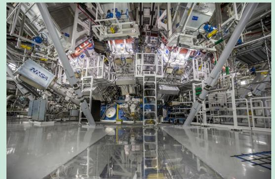
The target chamber of LLNL's National Ignition Facility, where 192 laser beams delivered more than 2 million joules of ultraviolet energy to a tiny fuel pellet to create fusion ignition on Dec. 5, 2022.
