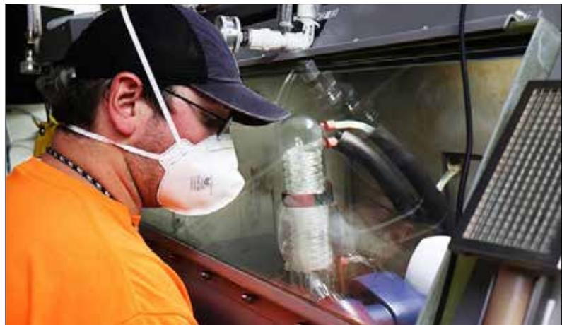
*Employees, known as fissile material handlers, use shielded gloveboxes to dissolve uranium (U)-233 into a low-level form so it can be mixed with grout for safe transportation and disposal.*
