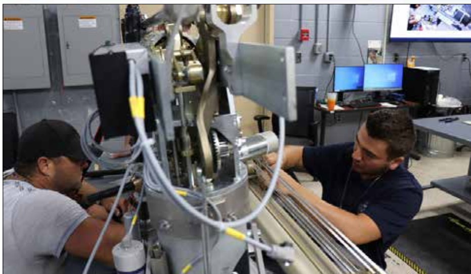
Isotek brought in a technical expert for two weeks to train millwrights on how to maintain and repair manipulators essential to the Uranium-233 Disposition Project.
