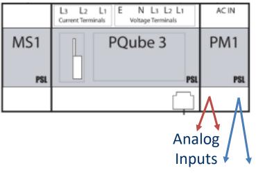
Power Input: 24VDC – 48VDC
