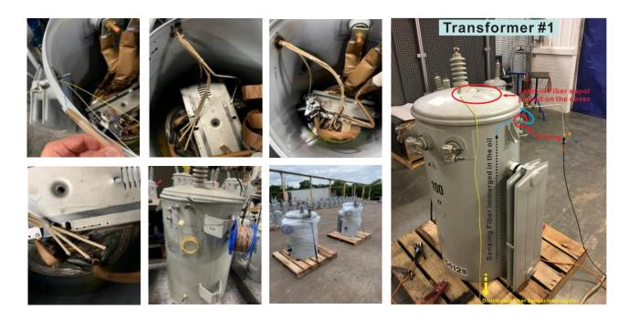
Three types of optical fiber sensors are integrated into operational distribution transformers for internal temperature monitoring during standard thermal runs.
