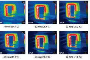
Standard IR-based thermal imaging measurement
