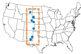
Existing dc links connecting eastern interconnection (EI), western interconnection (WI) ~ 1.0 GW transfer capability
