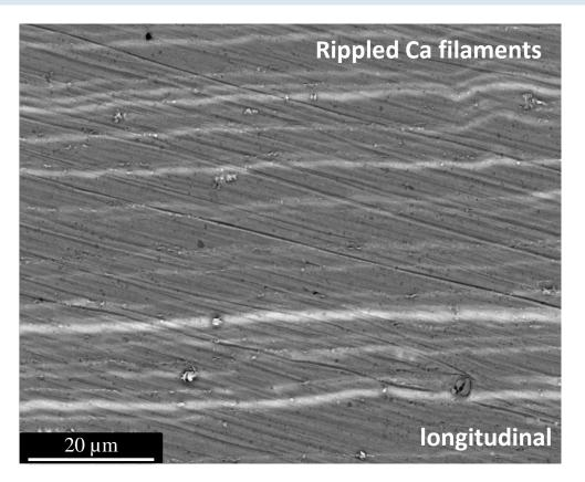
Smooth, continuous "drawing" deformation should reduce extruded billet to wire sizes with straight, stable Ca filaments.
