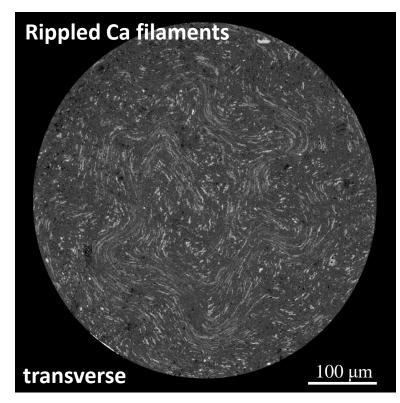
Initial deformation method (swaging) with opposing hammer dies produced rippled Ca reinforcement filaments.
