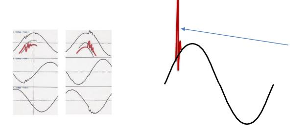
During Transient, frequency change/shift should be significantly above the steady state levels. Such difference from the steady state levels is the signal that we need to detect
