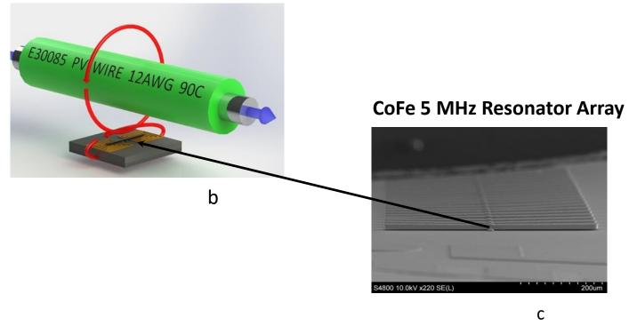
(a) and (b) illustration of Magneto-Strictive current sensing principle; (c) SEM photo of MagSense's magnetostrictive resonator
