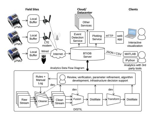
Detailed PMU system—output to grid components
