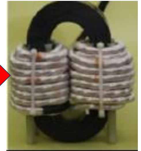
Full-scale Prototype Core w/ Nanocomposite Microstructure
