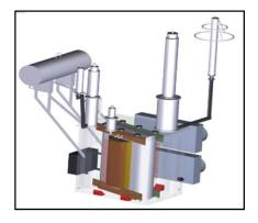
Beyond this solution, in order to accommodate flexibility of wide range of voltage (69 to 500 kV), and power (100 to 600 MVA), a further modular solution is necessary using the least number of modules possible to make it transportable using the utility trucks (<42 matric tons)</li>
