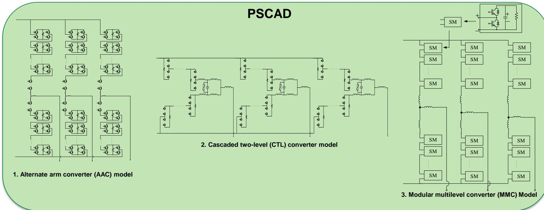
Fast Multi-level Voltage Source Converter (VSC) HVdc Converter Models
