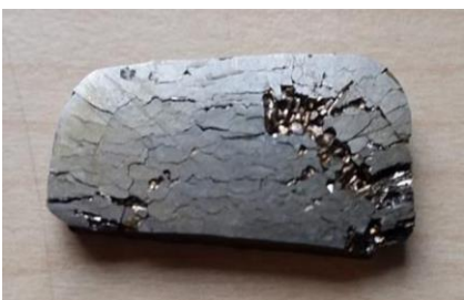
Cracking during rolling of Fe-6.5Si (Kustas, Purdue University, 2016)
