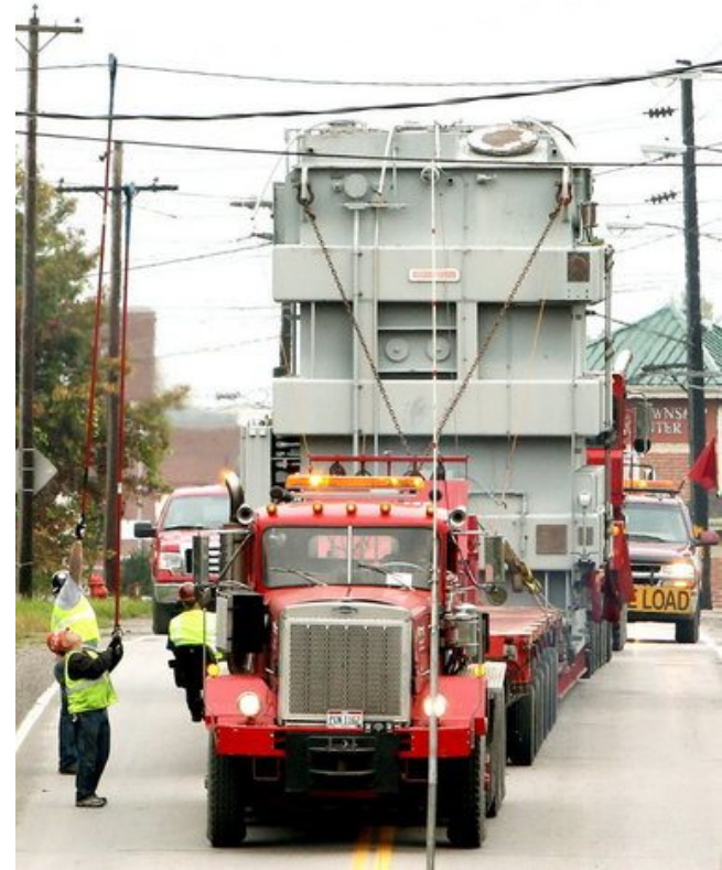
Transportation of a large power transformer.
