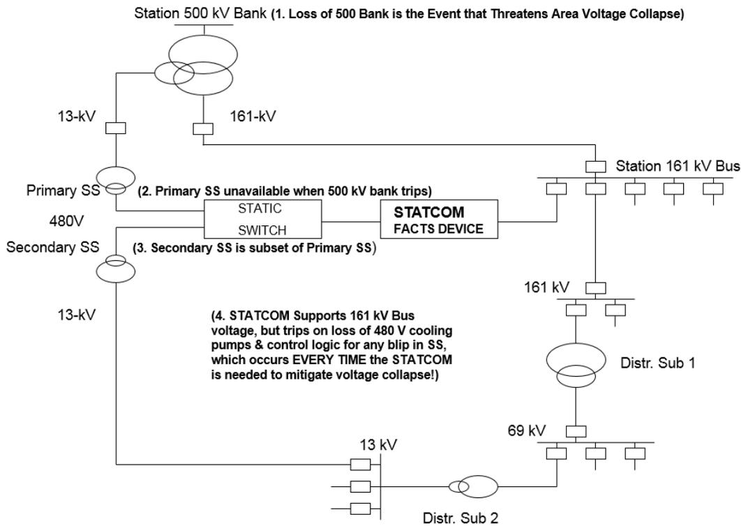
**Figure 3:** STATCOM Serial #1 Station Service – Still a common Achilles heel?
