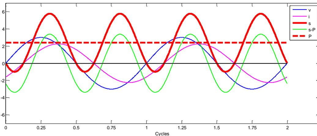
**Figure A-3.** Power in an AC circuit – general case.
