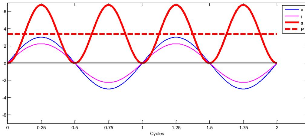
**Figure A-1.** Power in an AC circuit when voltage and current are in phase.
