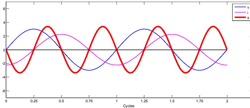
**Figure A-2.** Power in an AC circuit when current lags voltage by quarter of a cycle.
