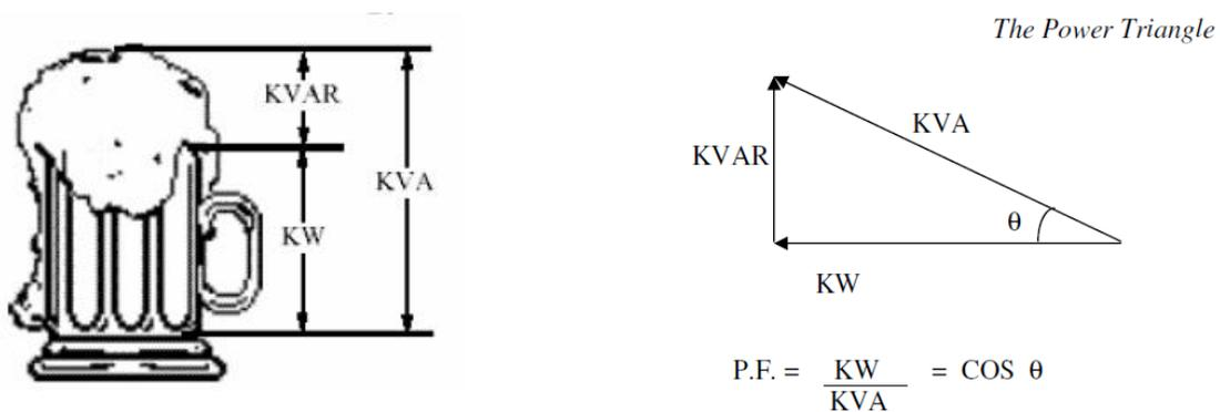
**Figure 2a and 2b.** Model of the beer analogy and the power triangle. Adapted from “Power Factor – The Basics,” by PowerStudies, Inc.
