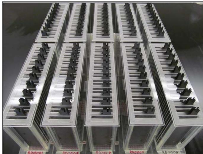
**Figure 65. 1-kW Zinc-air Prototype**
