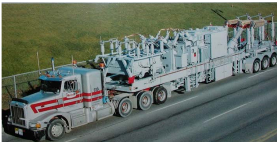
Figure 7. Mobile substation in transit.
