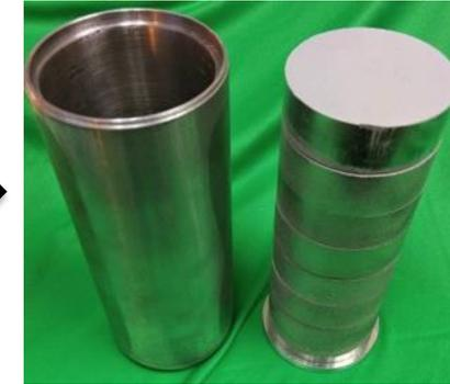
Extrusion can loaded with compacts
