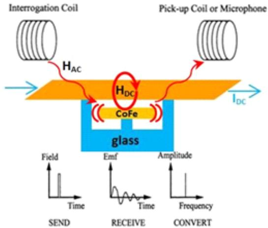
We developed a low-cost, frequency selective current sensor (MagSense), which allows observability of the state of health of grid components, detection of abnormal behavior/patterns of the components, and provides real-time detection of catastrophic failures.
