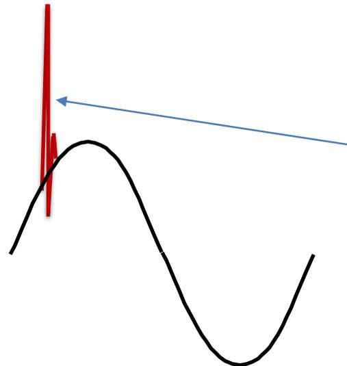
During Transient, frequency change/shift should be significantly above the steady state levels. Such difference from the steady state levels is the signal that we need to detect
