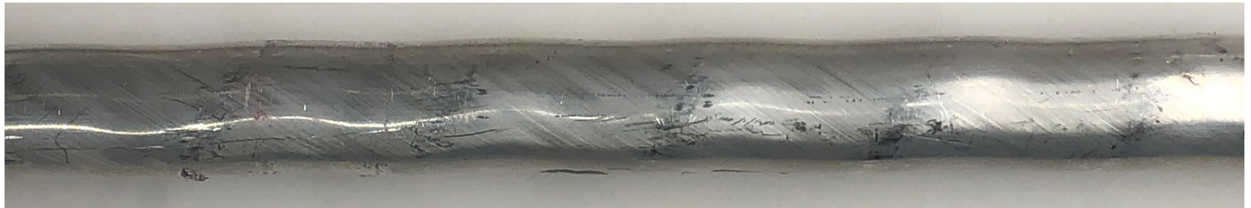
Baseline Tool: Twisted with rough surface
