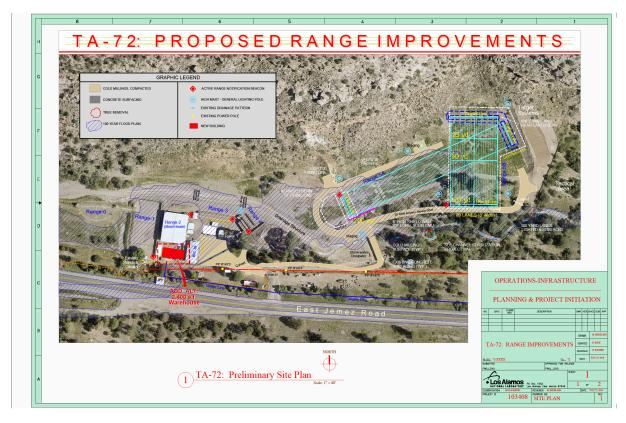
Figure 1. TA-72 Proposed Site Plan in relation to the 100-year floodplain.
