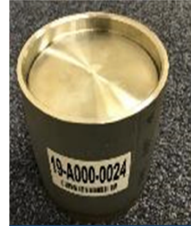
Lids are press-fit to close Robust Outer Container (ROC). ROC reduces radiation exposure for handling of Dilute Surplus Plutonium (DSP)
