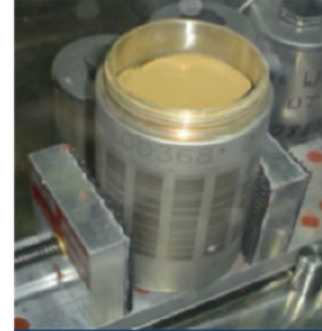
DOE-STD-3013 or alternate containers are opened for \text{PuO}_2 blending
