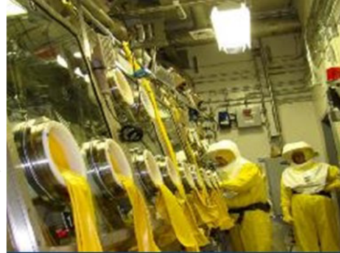
Plutonium oxide ( \text{PuO}_2 ) and Blend Can Kits are placed in a glovebox
