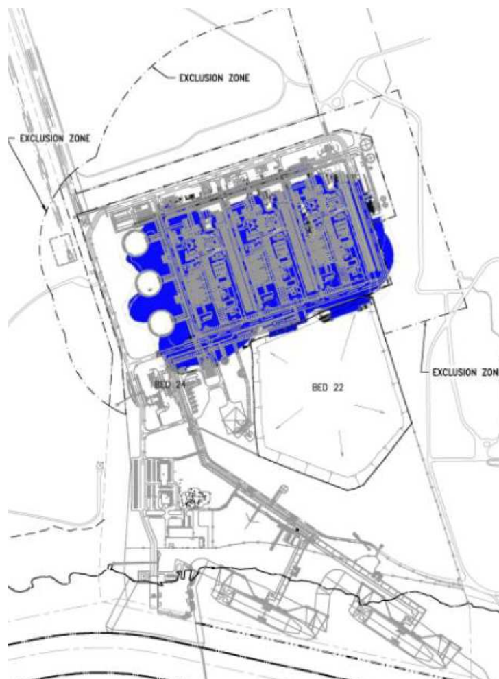
Figure 4.12-3 Vapor Cloud Explosion Overpressure Contours
