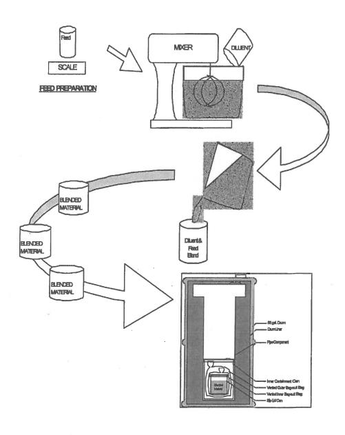
Figure 1. Schematic of Pipe-and-Go Process.
