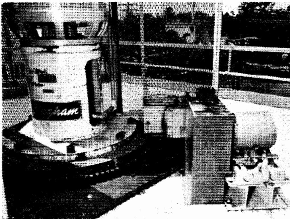
FIGURE C.9. Turntable and Pinion Drive for Slurrying Pump
